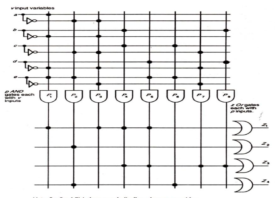
Note:  $5 \times 8 \times 4$  PLA shown symbolically and programmed for:  $Z_1 = p_1 + p_3 + p_4 + p_5 \therefore Z_1 = a\bar{b}\bar{d}e + \bar{a}\bar{b}\bar{c}\bar{d}\bar{e} + bc + de$   $Z_2 = p_2 \qquad \therefore Z_2 = \bar{a}\bar{c}e$   $Z_3 = p_4 + p_5 + p_7 + p_8 \therefore Z_3 = bc + de + \bar{c}\bar{d}\bar{e} + bd$  $Z_4 = p_2 + p_6 \qquad \therefore Z_4 = \bar{a}\bar{c}e + ce$
